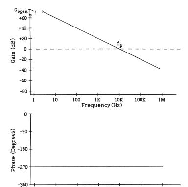
Figure B-16 The single-pole method of compensation.
