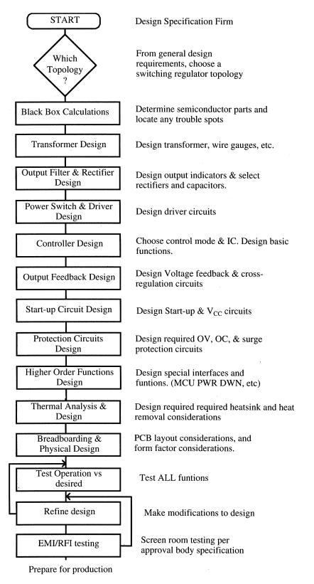
Figure 3–6 Design flow for a PWM switching power supply.
