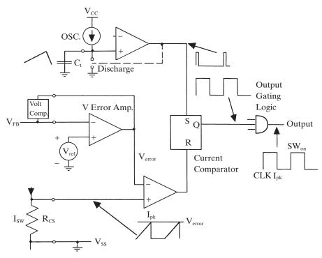
Figure 3-41 Turn-on with clock current-mode control.
