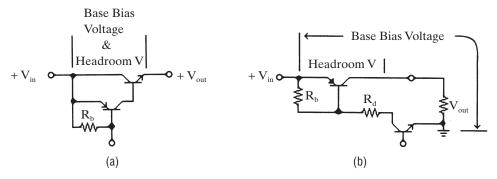
**Figure 2–2** The pass unit's influence on the dropout voltage: (a) NPN pass unit; (b) PNP pass unit (low dropout).
