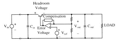
Figure 2–1 The basic linear regulator.
