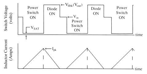
Figure 3-4 Waveforms for a discontinuous-mode boost converter.
