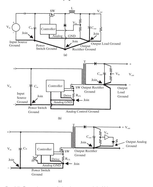
**Figure 3–61** The ground arrangements for the major converter topologies: (a) the nonisolated dc/dc converter; (b) the nonisolated, transformer-coupled converter; (c) the isolated, transformer-coupled converter.
