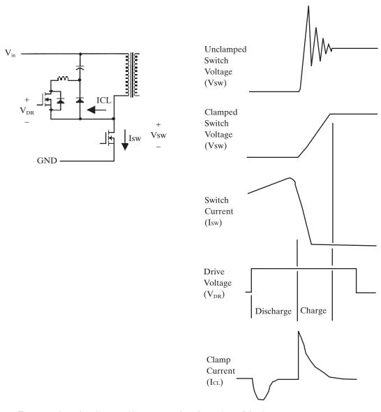
Figure 4–7 An active clamp used in a one-transistor forward or a flyback converter.
