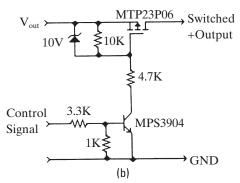
**Figure 3–58** Methods of switching power buses: (a) dual switching power supply with enable; (b) a dc power switch.
