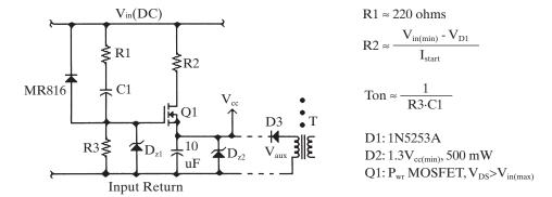
Figure 3-48 The overcurrent shut-down circuit.
