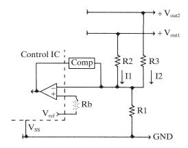
Figure 3-44 Multiple sense outputs.
