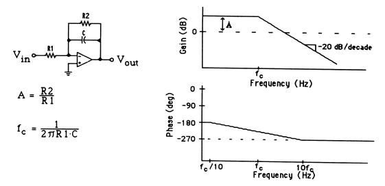
Figure B–6 An active single-pole filter with flat high- and low-frequency responses.
