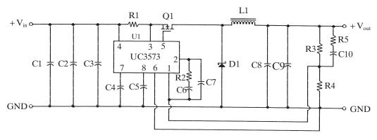
Figure 3-65 A 10-watt buck (step-down) converter.
