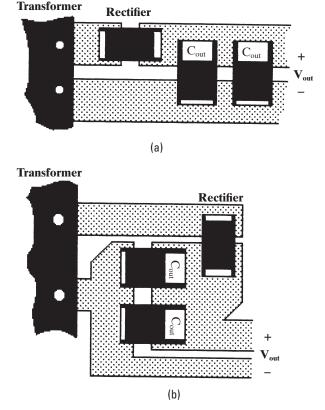
Figure 3–63 Laying out paralleled capacitors: (a) a poor layout for paralleled capacitors; (b) a better layout for paralleled capacitors.
