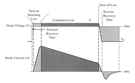
Figure 4-2 Rectifier losses.
