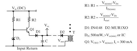
Figure 3-47 The high-voltage linear regulator bootstrap start-up circuit (used only at start-up and foldback periods).
