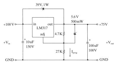
Figure 2-8 A high voltage floating linear regulator.
