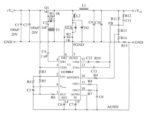
Figure 4-20 A 10 watt synchronous buck converter.
