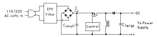
Figure C-4 A buck/boost power factor correction circuit.
