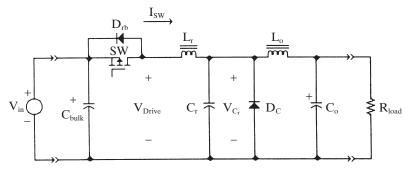
A. Schematic of a ZCS Quasi-Resonant Buck Converter
