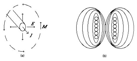
**Figure D–1** The fields around a conductor in free air: (a) field around a free wire; (b) field around a coil in free air.
