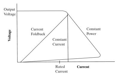
Figure 3-49 Types of overcurrent protection.
