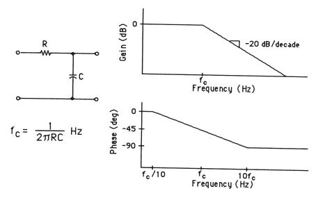
Figure B-1 A single-pole RC low-pass filter.
