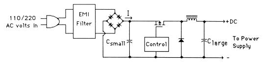
Figure C-3 A buck power factor correction circuit.
