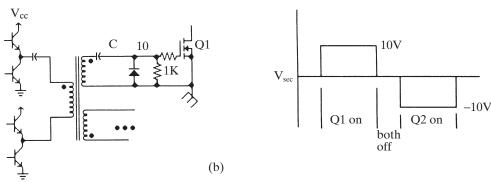
**Figure 3–23** Examples of transformer-coupled base and gate drives: (a) single MOSFET drive circuit; (b) dual MOSFET drive.
