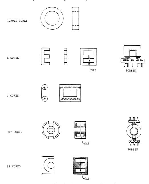
Figure D-6  $\,$  The common styles of magnetic cores.
