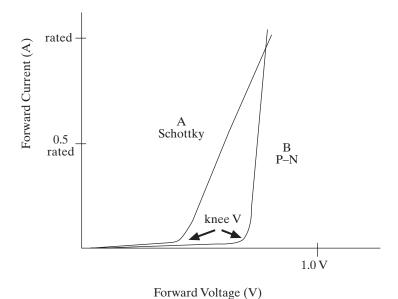
Figure 3–29 Forward conduction voltage characteristic of the Schottky versus the ultrafast diode.
