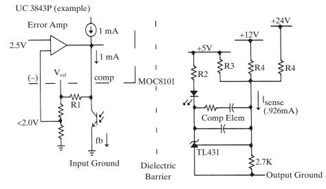
Figure 3-70 The voltage feedback circuit.
