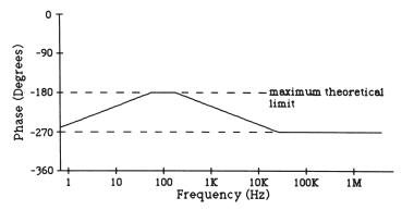
Figure B-20 The pole-zero compensation method.
