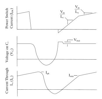
Figure 4–11 The schematic and waveforms of a ZVS quasi-resonant buck converter.
