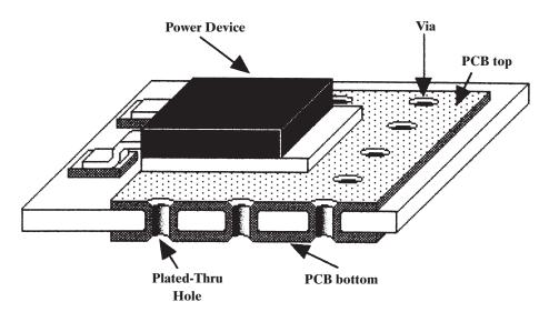
Figure 3–62 A good method for enhancing the heatsinking capabilities of a PCB island and minimizing capacitive coupling to other PCB traces.
