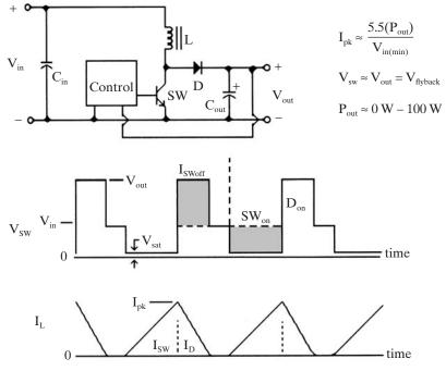
Figure 3-10 The boost (step-up) converter.
