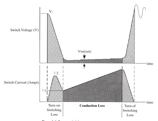
Figure 4–1 Power switch losses.
