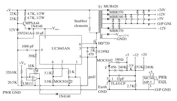
Figure 3–72 65 watt, off-line flyback converter.
