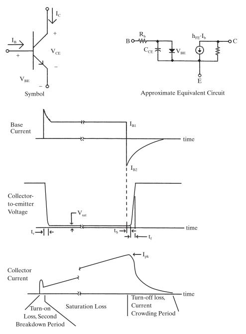
**Figure 3–32** Waveforms for a bipolar power transistor within a PWM switching power supply.
