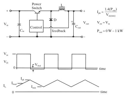
Figure 3-9 The buck (step-down) converter.
