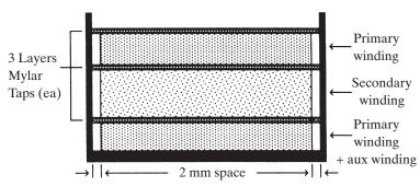
Figure 3–68 The transformer winding technique for design example 3.15.3.
