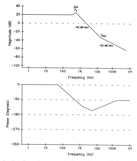
Figure B-11 The control-to-output curve for a forward-mode converter with voltage-mode control.
