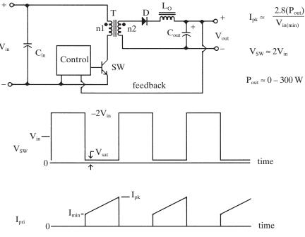
Figure 3–13 The one-transistor forward converter.
