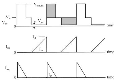
Figure 3-12 The flyback converter.
