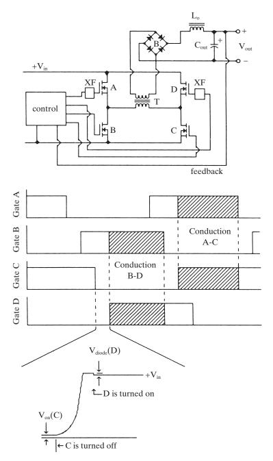
Figure 4–18 Phase modulation of a PWM full-bridge converter.
