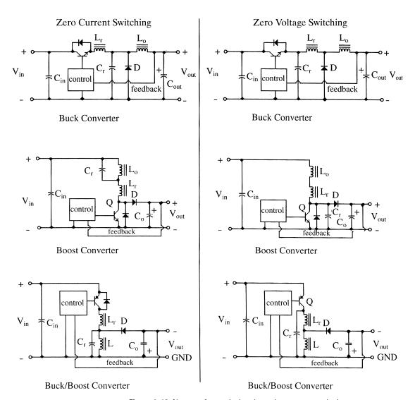
Figure 4–12 Nontransformer-isolated quasi-resonant topologies.
