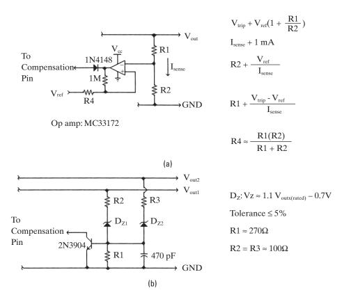
**Figure 3–53** Methods of overriding the voltage feedback loop in the event of its failure: (a) overvoltage override circuit (when voltage loop goes open-circuited); (b) multiple-output overvoltage override circuit.
