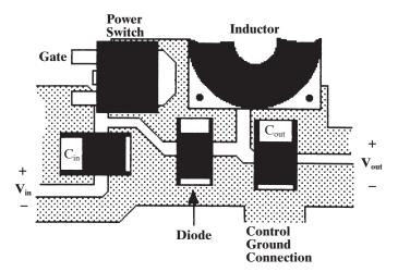
Figure 3-60 A good layout for a buck converter.
