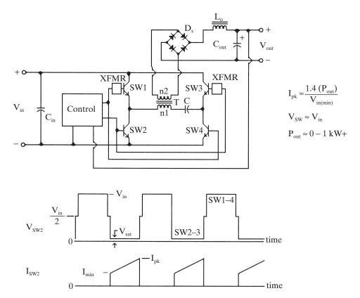
Figure 3-16 The full-bridge converter.
