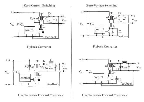
Figure 4–13 One transistor, transformer-isolated quasi-resonant topologies.
