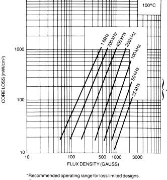
Flux density for bipolar excitation is B. Flux density for unipolar excitation is Bp-p.
