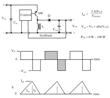
Figure 3–11 The buck-boost converter.
