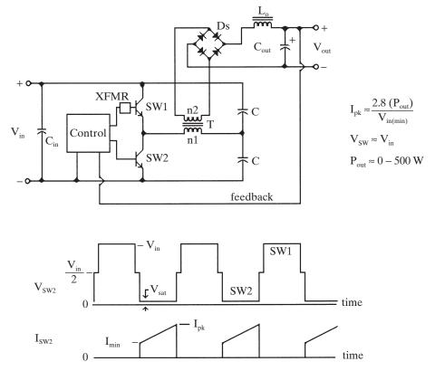
Figure 3–15 The half-bridge converter.
