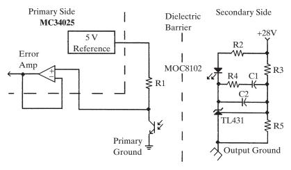
Figure 3-75 Voltage feedback arrangement.
