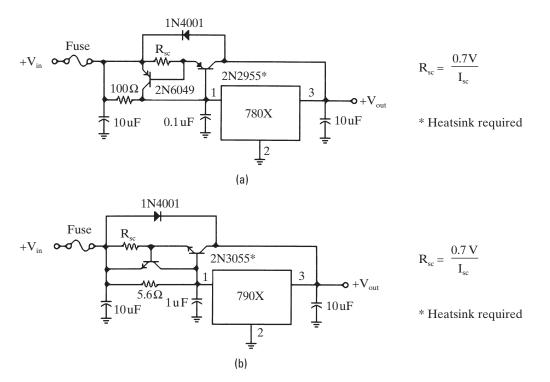
**Figure 2–7** (a) Positive current-boosted 3-terminal regulator with current limiting. (b) Negative current-boosted 3-terminal regulator with current limiting.
