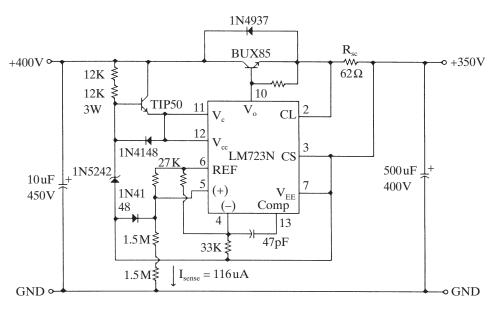
Figure 2-9 A 350 volt, 10 mA floating linear regulator.
