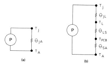
Figure A-6 The thermal model for an axial-leaded diode.
