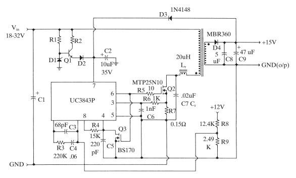
Figure 4-22 A ZVS quasi-resonant current-mode flyback converter.
