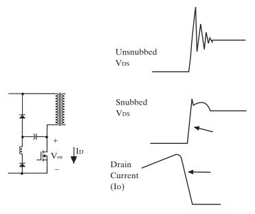
Figure 4–5 Lossless snubber for a one-transistor forward or flyback converter.
