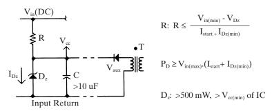
Figure 3-46 The Zener diode controller supply regulator.
