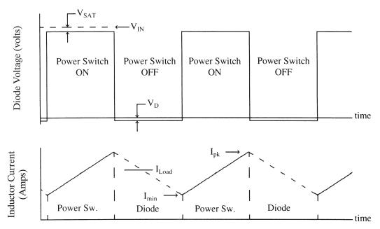
Figure 3-2 The voltage and current waveforms for a forward-mode converter (buck converter).
