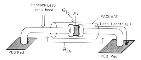
Figure A-5 Physical diagram of a mounted diode.
