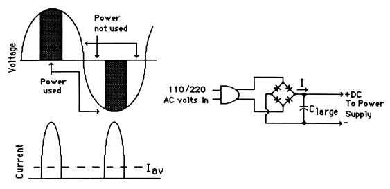
Figure C-1 The waveforms of a capacitive input filter.
