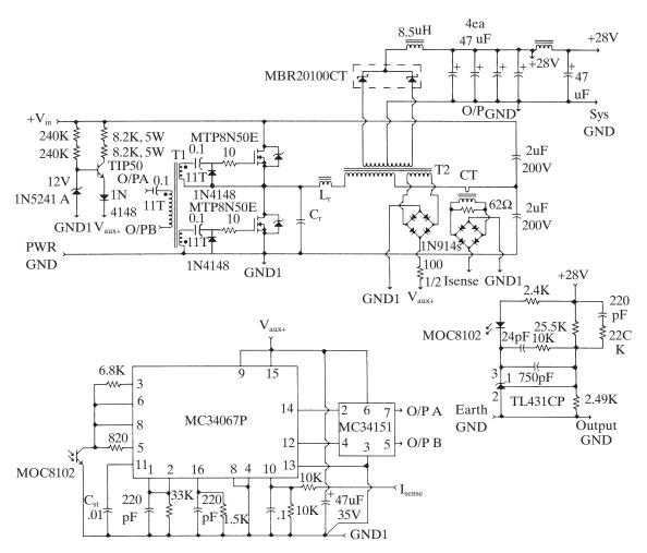
Figure 4-25 Schematic for the ZVS QR half-bridge converter.
