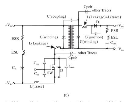
Figure 4–3 Major parasitic elements within converters: (a) buck converter; (b) flyback converter.
