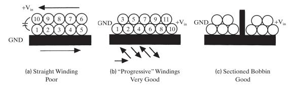
Figure 3–26 Winding technique for minimizing inter-turn capacitance.
