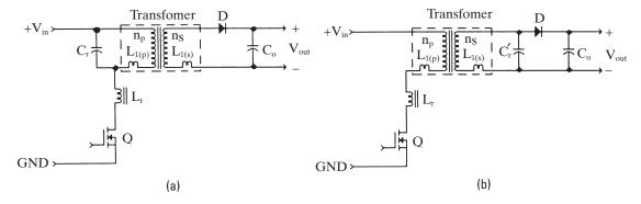
**Figure 4–16** "Pushing" the resonant capacitor through a transformer in ZCS ΩR supplies: (a) primary-side resonance; (b) secondary-side resonance.
