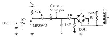
Figure 3-74 Current slope compensation pin.
