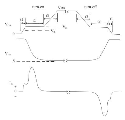
Figure 3–36 The MOSFET waveforms.
