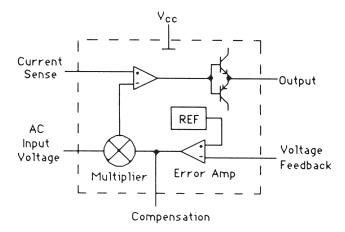
Figure C-6 A generalized typical power factor control IC.
