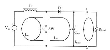
Figure 3–3 A basic boost-mode converter (boost converter shown).
