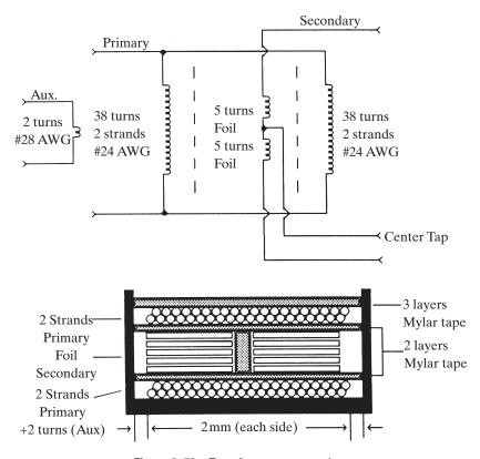
Figure 3–73 Transformer construction.
