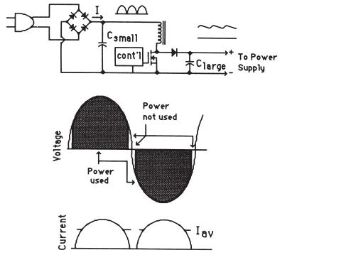
Figure C-2 Power factor corrected input.
