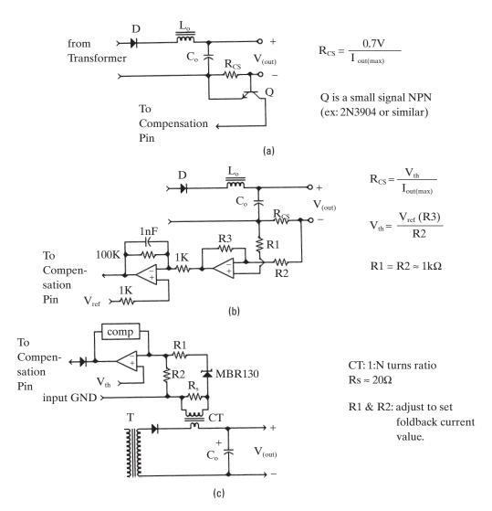
**Figure 3–50** Methods of constant current limiting: (a) discrete overcurrent limiting (constant-current limiting); (b) precision resistive current-sensing overcurrent protection (constant-current limiting); (c) use of a current transformer to sense ac current.
