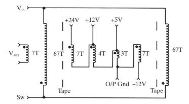
Figure 3–69 Transformer winding arrangement of design example 3.15.3.
