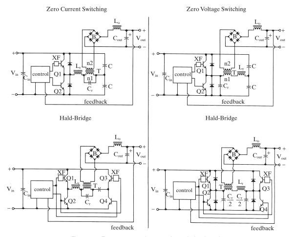
Figure 4–14 Two or more transistor, transformer-isolated quasi-resonant converters.
