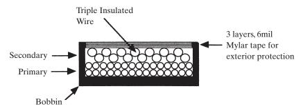
Figure 3–25 Off-line transformer using triple-insulated wire.
