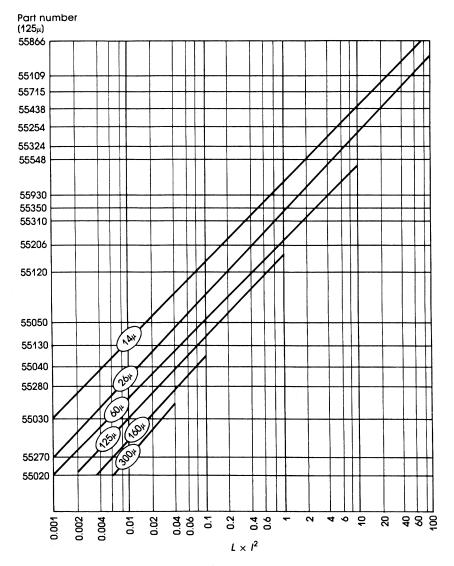
Figure 3–20 DC bias core selector chart (L = inductance with dc bias in millihenries; I = dc current in amperes) (Courtesy of Magnetics, Inc.).
