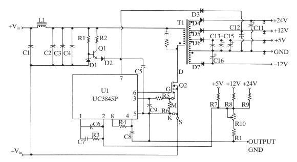
**Figure 3–66** Schematic for design example 3.15.2. A 28 W current-mode, flyback dc-to-dc converter.
