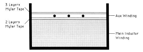
Figure C-8 Construction of the PFC boost inductor.
