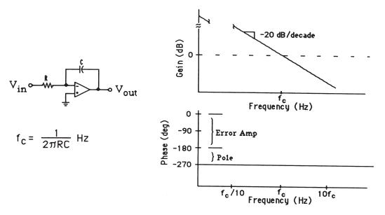
Figure B-5 An active single-pole filter.
