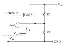
Figure 3-43 A nonisolated voltage feedback circuit.
