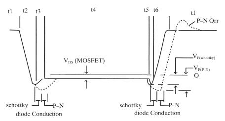
Figure 3–31 Critical time periods in the operation of a synchronous rectifier.
