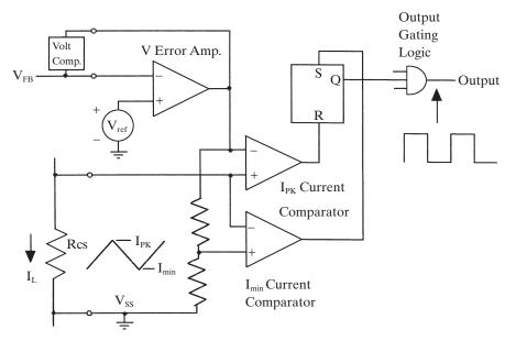
Figure 3-42 Example of hysteretic current-mode controller.
