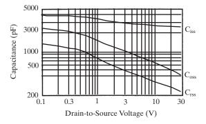
Figure 3–37 Representative datasheet curves for a MOSFET.
