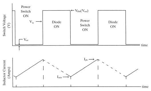
Figure 3–5 Waveforms for a continuous-mode boost converter.
