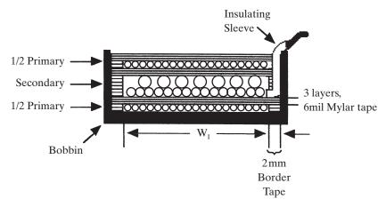
Figure 3–24 IEC-compliant, interleaved, off-line transformer.
