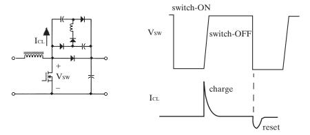
Figure 4–6 Lossless snubber for a boost converter.
