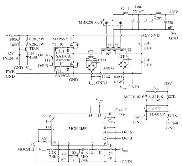
Figure 3–77 Schematic of a 100 kHz, 280 W, half-bridge converter.
