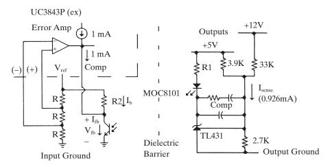
Figure 3-45 Example of an optoisolated voltage feedback circuit.
