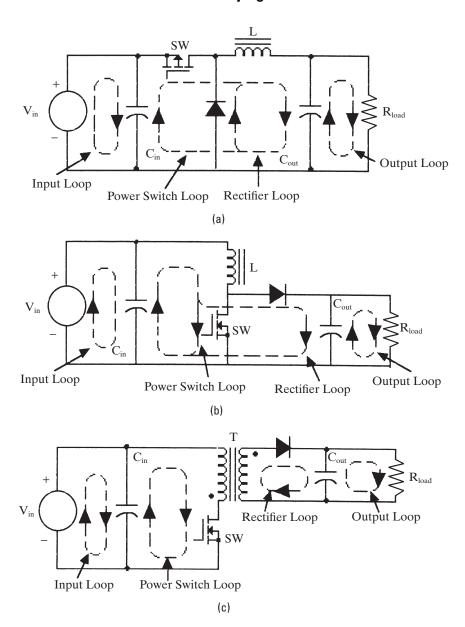
**Figure 3–59** The major current loops within the major switching power supply topology types: (a) the nonisolated buck converter; (b) the nonisolated boost converter; (c) the transformer-isolated converter.
