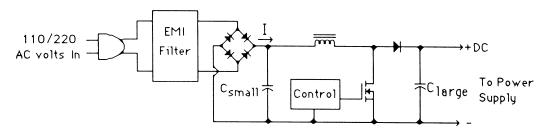
Figure C-5 A boost power factor correction circuit.
