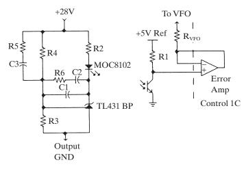
Figure 4-23 The voltage feedback circuit.
